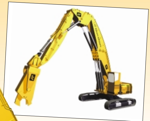
Main Picture: Dutch firm Rusch Special Products is currently modifying a Cat 5130 mining shovel into a 320-tonne demolition monster.
